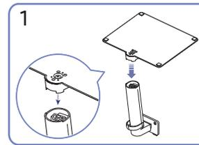
Put the stand base onto the stand neck as the direction shown in the figure. Check that the stand neck is firmly connected.
