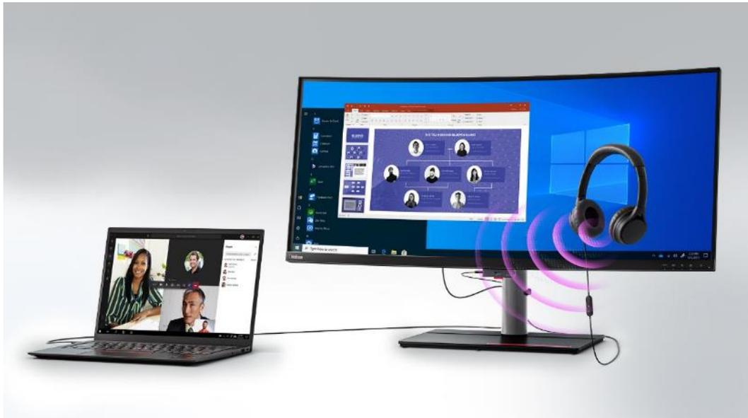
When plug off the earphone, the PC will not delivery the audio signal to monitor, it will delivery to other speakers connecting to PC. (internal or external speakers of PC)
